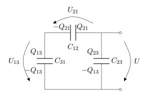
$$C_{12} = C_{21}, \quad C_{31} = C_{13}$$
