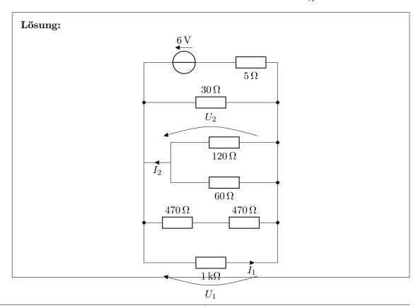
$$\frac{I_2}{I_1} = -\frac{1 \,\mathrm{k}\Omega}{120 \,\Omega//60 \,\Omega} = -\frac{1 \,\mathrm{k}\Omega}{40 \,\Omega} = -25 \tag{56}$$
