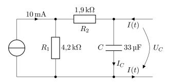
$$t = 0_{-} \quad I_{C} = 0, \quad I_{R_{2}} = 0$$
