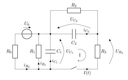
$$t = 0_{-}: I_{C_1} = I_{C_2} = I(t) = 0$$
