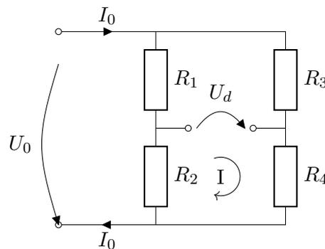
$$\text{I: } U_d + U_{R_4} - U_{R_2} = 0 \quad (13)$$
