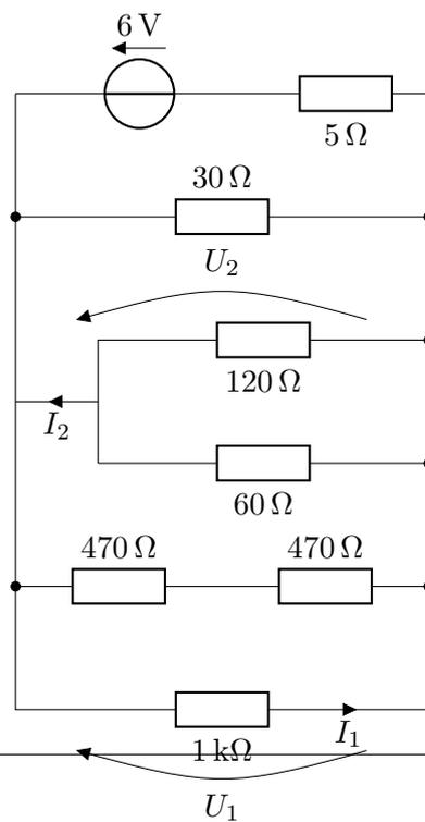
$$\frac{I_2}{I_1} = -\frac{1 \text{ k}\Omega}{120 \Omega // 60 \Omega} = -\frac{1 \text{ k}\Omega}{40 \Omega} = -25 \quad (12)$$
