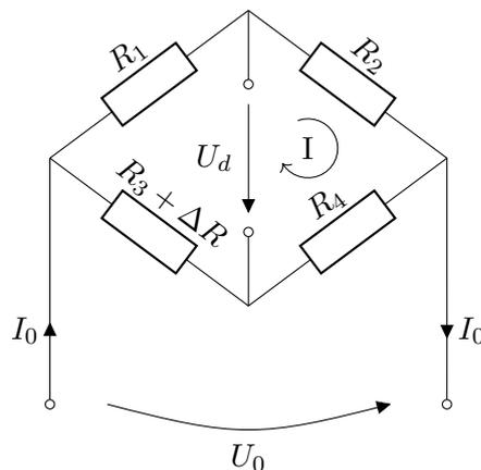
$$\text{I: } U_{R_2} - U_{R_4} - U_d = 0 \quad (21)$$
